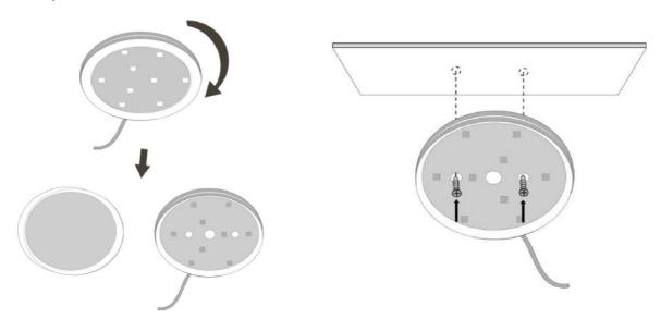
Pic.2 Installation with screws
