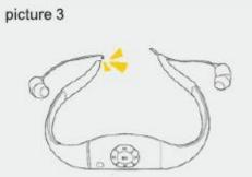
The copper wires of the headphone cables will be broken and headphone no sound, see picture3
