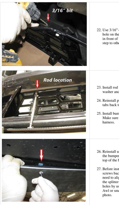
22. Use 3/16" drill bit to drill a hole on the bumper skin just in front of the grill. Repeat step to other side.
