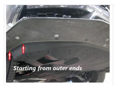
28. Reinstall factory screws back to the under-tray. You want to start from the outer end and work your way to the center section
