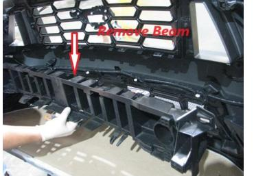
20. Remove plastic reinforcement beam on the bottom of the grill.
