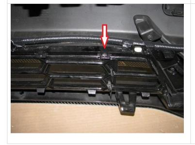
21. On each end of the grill, you should see a metal screw on it. Right in front of this screw is where you need to drill a hole for support rod to attach.
