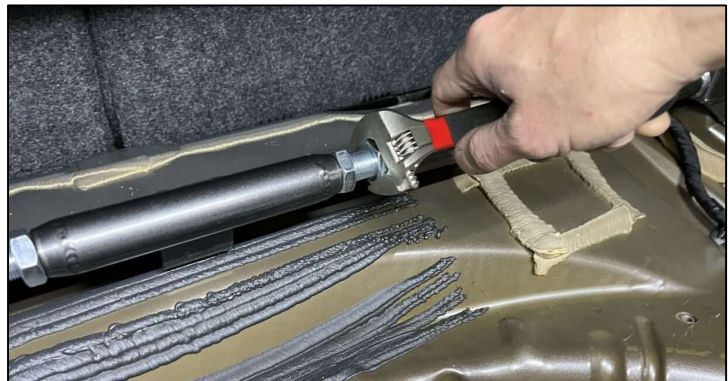
Tighten the Jam Nuts at the end of Installation
