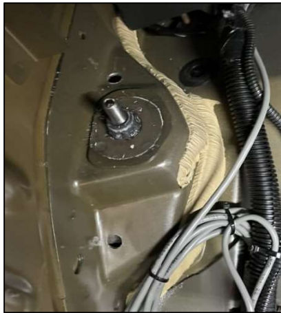
Drilled Holes on Shock Towers
