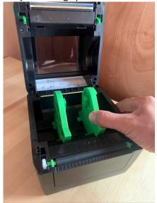
Install the roll, so the label is on the top (and you are looking at the label)
