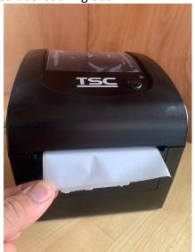
Push the feed button on the lid – and the machine will detect the labels and move to the start of the next label:
