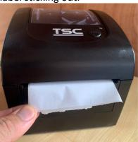
5. Push the feed button on the lid – and the machine will detect the labels and move to the start of the next label:
