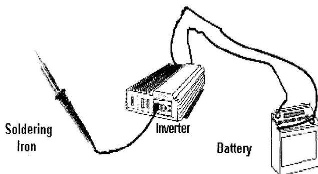
The adhesives, three different butane-powered soldering irons, and one battery-powered soldering iron were evaluated in 2007, and the 25-watt electric soldering iron/voltage inverter/automobile battery was evaluated in 2008. The automobile battery was recharged following each banding session by attaching it to a battery charger (Deltran Battery Tender Plus; Deltran Corporation, 801 US Highway 92E, Deland, FL 32724) overnight.
