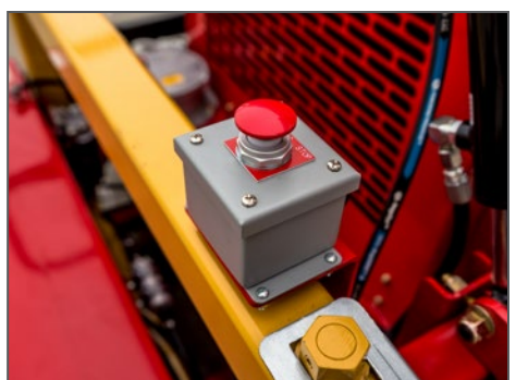
EMERGENCY STOP Maximum safety with five Emergency Stop Push Button Switches, plus Horn and Strobe
