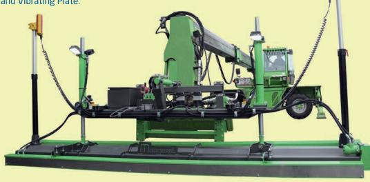
The **MS40** attachment is completely automated, offering high production output with superior accuracy at 4.2m (14ft) wide, it features a plough, auger, roller and vibrating beam for ultimate compaction. It is very easy to operate via a wireless 7" colour touchscreen display, with full visualisation allowing the operator to fine tune and make adjustments for easy operation. Made in Belgium.
