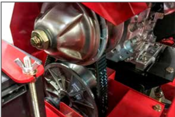
The torque convertor clutch ensures maximum control over machine speed.
