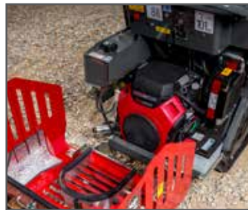
Engine cover folds back to provide convenient access to the engine, gasoline tank, battery, and filters.
