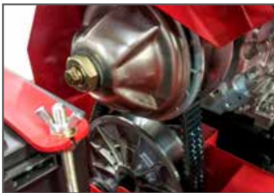
The torque converter clutch ensures maximum control over machine speed.
