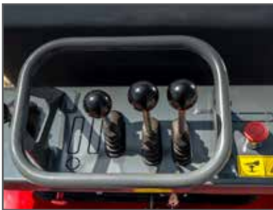
Two servo levers control the direction of the machine, and they automatically reset to stop in case of emergency.
