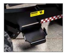
Side-to-side and rear-tofront forklift pockets provide convenient loading options.
