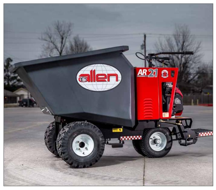
The twenty-one cubic foot AR21 comes standard with a high-strength, high-density polyethylene bucket that provides excellent durability. It also comes equipped with features like heavy-duty hydraulic wheel motors, steel raceways for hydraulic hose protection and foam-filled tires ensure the AR21 power buggy will operate for the duration under even the toughest of conditions.
