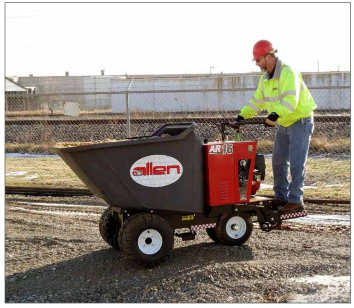
The sixteen cubic foot AR16 has earned it's rank as the standard by which all power buggies are judged. The standard high-strength, high-density polyethylene bucket is the industry's thickest and most durable. Standard features like heavy-duty hydraulic wheel motors, steel raceways for hydraulic hose protection and foam-filled tires ensure the AR16 power buggy will operate for the duration under tough conditions.
