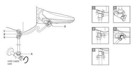
Please turn on the water supply valve and check connected spots (1-5) for the leakage.
