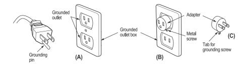
4. If it is necessary to use an extension cord, use only a three wire extension cord that has a three-blade grounding plug, and a three-slot receptacle that will accept the plug on the product. Do not use a damaged extension cord.
