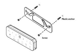
Fasten the remote control bracket with double sided adheasive tape on the proper area of the wall as shown.
