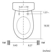
The toilet dimensions must be within those shown above. Do not install this appliance on a toilet that does not meet those dimensional requirements.
