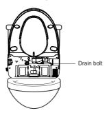
• Unscrew the mounting bolts. Refer to the installation procedure.
