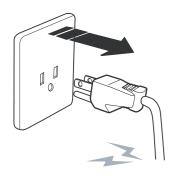
Unplug the power supply cord. Not doing so may cause electric shock or fire. 2. Close the shutoff valve.
