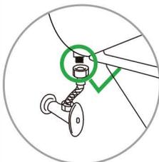
Inspect your current water supply line that connects to the toilet tank fill valve to ensure it is a flexible water supply hose. If it is a rigid pipe, you will need to purchase a flexible water supply hose before installing the SlimGlow. The hose needs to be 7/8" (to connect to the T-valve we provided) on one end and either 3/8" or 1/2", depending on your wall valve, on the other end.
