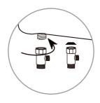
4. Connect the 7/8" T-Valve to the toilet fill valve where you just removed the water hose from.
