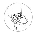
8. Place the circular mounting brackets into the bidet attachment.
