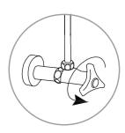
12. Slowly turn the water supply valve back on, check for leaks, and test the unit for functionality.
