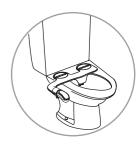
10. Place the toilet seat back on the toilet over the bidet and secure the bolts down so that the seat and bidet attachment are stable.
