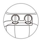
9. Place the bidet on the toilet with the mounting brackets over the mounting bolt holes and make any needed adjustments to make sure the bidet is centered on the toilet and so you can see the mounting bolt holes through the mounting brackets of the bidet.
