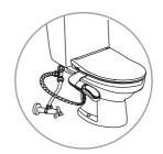
11. Connect the hose from step 6 to the bidet water connection underneath the handle of the SlimTwist.
