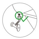
Please be advised that the provided T-Valve should be installed at the fill valve under the toilet tank, NOT down at the water supply coming from the wall.
