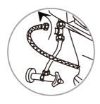
6. Connect the metal hose we supplied to the open side of the T-Valve.
