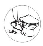
11. Connect the hose from step 6 to the bidet water connection underneath the handle of the SlimGlow.
