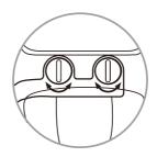
9. Place the bidet on the toilet with the mounting brackets over the bolt holes and make any needed adjustments to make sure the bidet is centered on the toilet.
