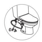
11. Connect the hose from step 6 to the bidet water connection underneath the handle of the SlimEdge.
