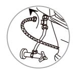
6. Connect the metal hose we supplied to the open side of the T-Valve.
