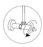
12. Slowly turn the water supply valve back on, check for leaks, and test the unit for functionality.
