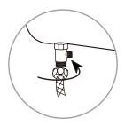
5. Attach the water supply hose that comes from the water shut off to the bottom of the T-Valve.
