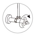
2. Close the water supply valve and flush the toilet completely so that there is little to no water left in the toilet tank
