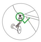
Please be advised that the provided T-Valve should be installed at the fill valve under the toilet tank, NOT down at the water supply coming from the wall.
