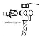
Remove protective plastic covers on threaded caps from the ends of the 48" stainless steel supply hose. Attach the hex-head end of the hose to the T-valve.
