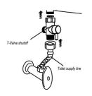
• Attach the 7/8" T-valve shutoff to the threaded fill valve on your toilet. Be sure the 7/8" flat washer is in the T-valve before installing. Position the T-valve so that the shuttoff handle is facing the front of the toilet.
