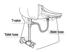
\*Do not overtighten connections.
