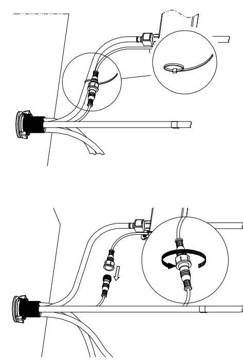
**7.** Install the counterweight on the pulldown hose at the marked position (It should be placed on the line).
