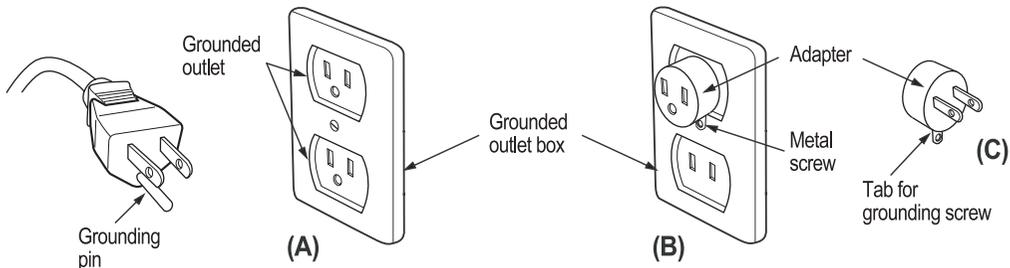
4. If it is necessary to use an extension cord, use only a three wire extension cord that has a three-blade grounding plug, and a three-slot receptacle that will accept the plug on the product. Replace or repair a damaged cord.
