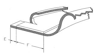
Compound placement may extend up to the cut edge at a given point but should not exceed .50 inch total length along the cut edae.
