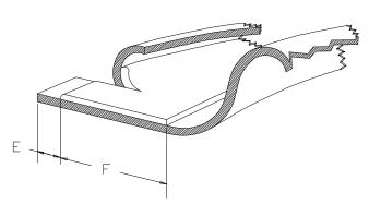
Compound placement may extend up to the cut edge at a given point but should not exceed .50 inch total length along the cut edge.
