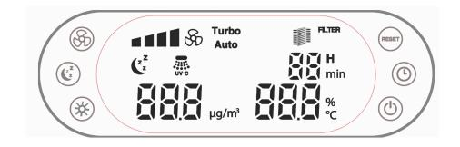
**5-Fan Speed:** Press this button repeatedly to select the desired fan speed. In Turbo mode, the unit runs for 15 minutes with UV lamp
