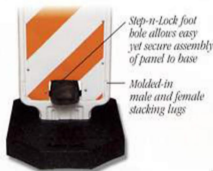
24" x 8" TrafiX Vertical Panel Barricade with light and 43lb. recycled rubber base 34000 Series
