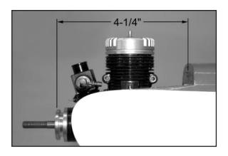
□ 39) Now set your engine aside and unbolt the engine mounts from the firewall. Drill clearance holes for your engine mounting bolts all the way thru the engine mount beams at the four locations you marked in the previous step. TIP: Secure the engine mounts in a vise while you drill the holes. If at all possible use a drill press instead of a hand drill - the job will be much easier and the holes will be straighter.
