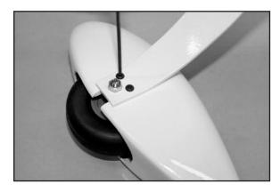
☐ 10) Using three M4 x 20mm Socket-Head Bolts and three M4 Flat Washers, bolt the landing gear onto the fuselage.
