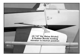
c) Inside the fuselage, hold the pushrod wire over the elevator servo output arm and mark the wire where it crosses over the outer hole in the servo arm.
