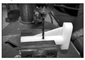
IMPORTANT: DO NOT USE ANY TYPE OF SCREW TO MOUNT YOUR ENGINE TO THESE MOUNTS. ALSO, DO NOT DRILL AND TAP THESE ENGINE MOUNTS FOR BOLTS! Doing so may weaken them and cause failure. Mount your engine to these mounts with steel bolts with flat metal washers and nylon insert lock nuts. Drill clearance size holes for the bolts completely through the mount beams. The mounting bolts should go through the holes without binding.
