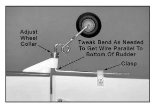
the clasp a little over halfway back on the wire, and then drill a hole for the M2 x 15mm Bolt. Insert the bolt through the hole and tighten down the M2 Hex Nut to clamp the bracket in place.
