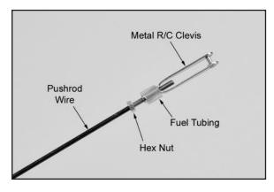
b) Locate the pre-cut pushrod exit hole for the elevator on the right side of the fuselage at the back of the plane. Slide the pushrod into the exit hole and inside the pushrod sleeve built into the fuselage. Slide it in until you can clip the clevis into the middle hole of the control horn. Lock the elevator in neutral position with tape, or with two small balsa wood sticks held together with small rubber bands.
