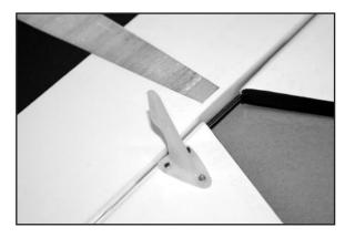
□ 13) Bolt the wing in place on the fuselage with the Nylon Wing Bolts provided. Then pin the stabilizer and elevator assembly in place on the fuselage. It's time to check the alignment of the stabilizer to the wing.
