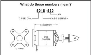
NOTE: This numbering system is very common, however there are exceptions. For instance, some motor manufacturers will list the actual diameter of the stator (armature) inside the motor instead of the case diameter. Some may list the length of the stator inside the motor instead of the case length. Some will give you both if you dig far enough into their specs. Make sure you understand the motor manufacturer's numbering system when shopping for a motor.
