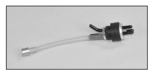
c) Once you are satisfied with the fit of both the fuel clunk line and the vent line you can tighten the machine screw to expand the rubber stopper and seal the stopper in the tank. Do not over tighten the screw as it can cause the tank to split. Attach three 6-inch lengths of silicone fuel tubing (not furnished) to the tank and label them appropriately as FILL, CARB, and VENT so you can identify them after the tank is installed in the airplane.
