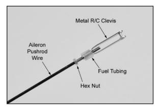
b) Clip the metal clevis into the last hole in the nylon control
