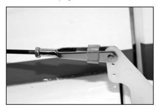
□ 25) Locate the pre-cut pushrod exit hole for the rudder on the left side of the fuselage at the back of the plane and repeat step 24) in its entirety to install the rudder pushrod.
