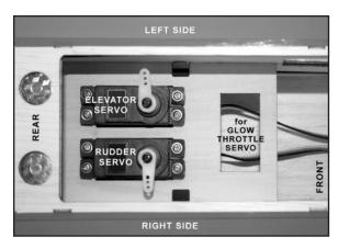
□ 23) Figure out where and how to mount your receiver. This can depend on several factors, starting with whether you are using a glow engine or an electric motor for power. We decided to mount the receiver of our photo model, which will be electric powered, on the left side of the fuselage, using a short piece of common Velcro® tape (not furnished).
