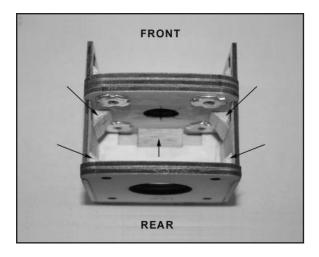
□ 30) Install your ESC now, before mounting the motor permanently. Note that ESCs can vary a lot in size and shape, so it is difficult to give "one size fits all" instructions on the best mounting location and method. This step describes how we mounted our Castle Creations 75A ESC in the top of the nose, which still left plenty of room for the lipo battery pack below the ESC.
