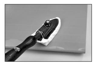
After you have all the covering secured onto the solid areas, turn the temperature of the iron up to approximately 300°F - 320°F (149°C - 160°C). This is the correct temperature for shrinking the covering material.
