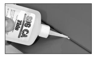
e) Turn the part over and glue the other side of the hinge. Continue this process until you have glued both sides of all the hinges! Keep a rag handy to wipe off any excess Thin CA glue. (If you get some glue smears on the plastic covering, don't worry about them right now. Once all the hinging is done, you can clean the smears off the covering with CA Debonder).
