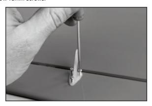
When the tips of the screws begin to emerge at the top surface of the aileron, add the control horn's nylon retaining plate. The aileron will be sandwiched between the control horn on the bottom and the retaining plate on the top. Continue turning in the screws until the horn and retaining plate are snug against both surfaces of the aileron. Do not over tighten the screws and crush the wood.
