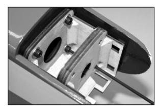
□ 32) If you have not already re-attached the X mount plate to the back of your motor, do so now. Then use (4) M4 x 16mm Socket-Head Mounting Bolts and Lock Washers to bolt your motor in place on the plywood motor mount box.
