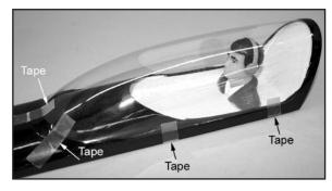
**WARNING:** Do not use thin CA glue to attach the canopy because it can cloud the plastic.
