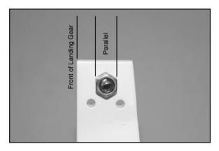
☐ 6) Slide a 4mm Wheel Collar onto the axle shaft, but leave approximately 1/8" of space between it and the nut, to provide proper spacing of the wheel in the wheel pant. Tighten the wheel collar set screw securely.
