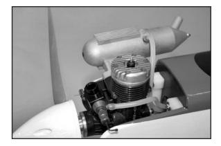
If you do elect to use the cowling, large openings will need to be made in the cowling to clear the engine cylinder head and muffler, and to allow access to the needle valve, etc. Don't be tempted to quickly dive in with a knife and start removing large chunks of material. You will achieve a lot better result if you take the time to develope a pattern and mark it on the cowling for guidance when you are cutting.
