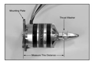
☐ 27) For the Somethin' Xtra, you need a distance from the back edge of the motor mount to the motor's thrust washer to end up
