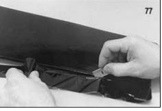
Using your hot sealing iron, carefully iron the covering material from the center of the wing panel out towards the wing tip, and then out towards the wing root. This is to help avoid trapping air bubbles under the covering. Work slowly and allow the iron to shrink the covering as you go along. Trim the covering off flush with leading edge and reseal it with the iron.
