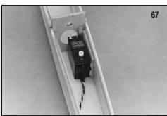
BUILDER'S TIP: Apply a thin coat of slow C/A to the balsa spacer and allow the glue to dry before taping the servo in place. This will greatly increase the bond of the servo tape. The remainder of the elevator pushrod installation details will be done later during "Final Assembly", after the tail surfaces are mounted to the fuselage.
