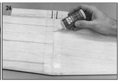
An alternate method of attaching the glass tape is to lightly spray one side of the tape with a spray adhesive (such as 3M "77"). Place the tape on the wing joint (sticky side down) and smooth out any wrinkles. Soak the glass tape with thin C/A.
