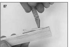
88. Cut out the sheeting from the center section for the aileron servo. The exact size of the opening will depend on the particular brand of servo and the method of mounting.
