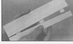
Place three or four drops of any brand of cyanoacrylate adhesive (thinnest variety) directly onto the Easy Hinge in the gap. You will notice that the glue is quickly wicked into the slot as it penetrates both the wood and the hinge. Continue this process, gluing the same side of all of the hinges. Then turn the surfaces over and repeat the gluing process on the other side of each hinge.
