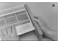
25. Trial fit the aileron to the torque rod. Once it fits, temporarily tape the aileron in place and sand the outboard end flush with the wingtip.
