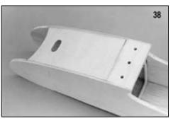
39. The fuselage is now ready for final sanding. Sand off all "Tee-Lock" tabs then round the bottom edges of the fuselage and the corners of the balsa top deck. Use a sanding block, starting with 80-grit sandpaper. Switch to 150-grit or 220-grit sandpaper for the final sanding.
