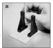
27. Lightly hammer four 6-32 blind nuts into the back of F-1. Bolt the engine mounts to the front of F-1 using 6-32x3/4" mounting bolts to align the blind nuts (see note below). Apply medium or slow CA around the edges of the blind nuts to hold them in place. Be careful not to get any glue in the threads.
