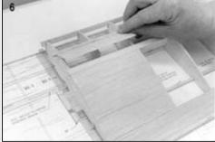
7. When the glue has dried, unpin the wing half from the board and install the 3/16"sq.x30" balsa bottom forward spar.
