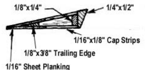
Aileron Rib Cross-Section
