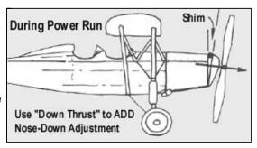
It's not likely that your plane will dive on first power flights, but if it should, put the shim at the bottom of the noseblock, tipping the propeller upward (upthrust).
