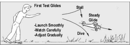
Begin by gliding the model from your hand into a patch of tall grass. Grasp the ship by the fuselage near the balance point, and aim the nose at a spot on the ground about twenty feet in front of you. Launch the ship forward about the way you would a paper dart airplane, nose down.
