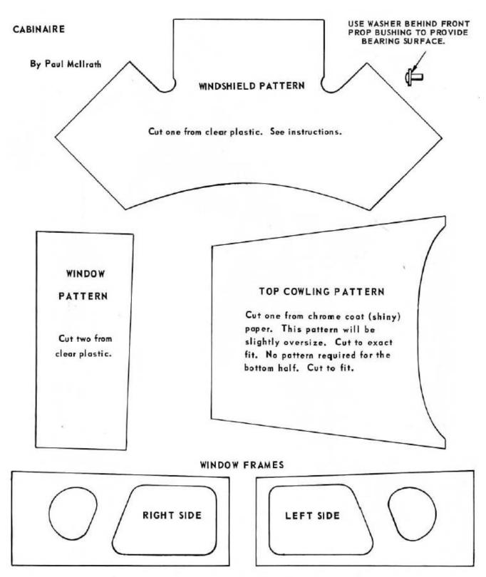
Cut two window frames, one right and one left, from this sheet or from typewriting paper
