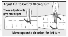
Small changes in fin setting can be made by bending the surface. But if more than 1/32" or so of change is required, cut the fin loose and re-cement it at the desired angle. When the glide is smooth and steady, you are ready to go on to powered tests.
