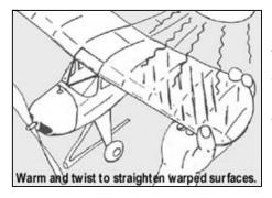
A model can be made to fly with twisted surfaces, but it's confusing to adjust and if the warps change from day to day, you can't detect it. The drawing shows how a surface can be straightened by twisting it in the desired direction while holding it under a heat lamp or other electric heater. Work with it until it is as flat as possible. If your wing has struts, loosen them before bending and re-cement them afterward.
