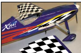
Two-Piece Wing With Super Strong Aluminum Wing Joiner Tube. Factory Painted Wheel Pants.
