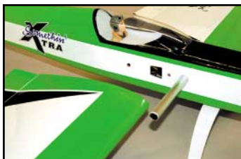
Two-piece Wing Design With Super Strong Aluminum Wing Joiner Tube. Easy To Transport & Easy To Store.
