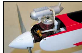
"EG" Means It Can Be Flown With Glow or Electric Power. Typical 2-Stroke glow engine installation.
