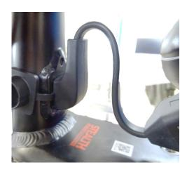
Connect the bridge cable to the frame plug as the picture shows. If the bike is equipped with a rubber band, that will help to keep the plug and connector together.
