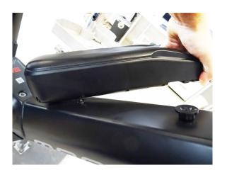
Slide in the battery, first from below bracket and turns the battery clockwise to clamp the top bracket from the left side of the main tube.
