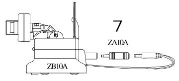
8. Turn the switch on the side of the ZB10A on. Turn off when not in use (4 hour battery life). Refer to the setup and operating instructions that came with the XCam II camera system for camera setup and operation.
