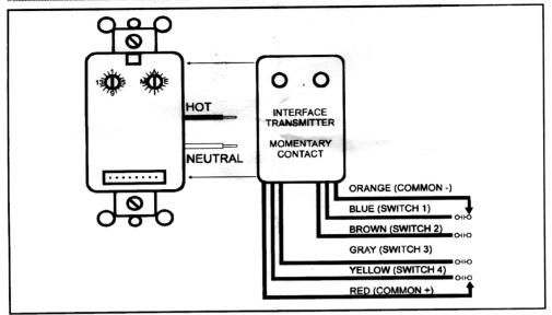
The XPT3 Interface Transmitter is a wall mounted controller capable of transmitting from a standard, single gang wall box having HOT and NEUTRAL.
