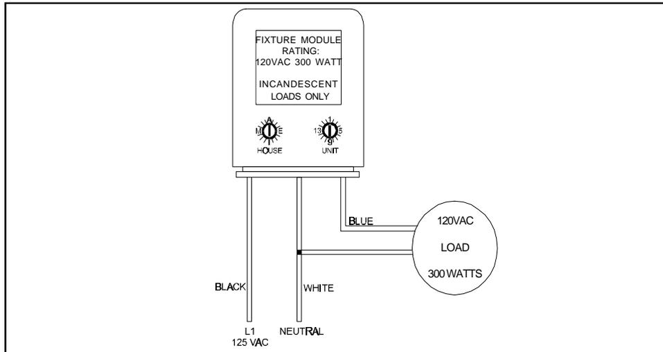
The XPDF Incandescent Dimmer Fixture is designed to control Incandescent loads of up to 300W. The XPDF is small enough to fit inside recessed lighting cans and single gang boxes of new or existing loads, allowing hard wired control from inside the fixture.
