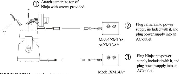
\* IMPORTANT! Do not interchange power supplies. Model XM14A must be used only for the Ninja Pan 'n Tilt base.
