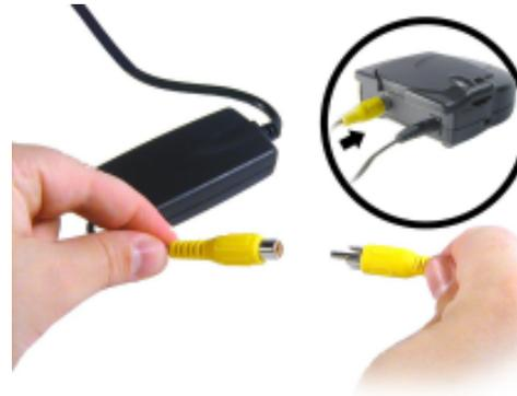
If you are using the Video Converter with a wired X10 camera like Anaconda or NightWatch, connect the video output of the camera directly into the yellow video input on the Video Converter.
