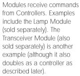
Controllers are also plugged into standard wall outlets and send commands to Modules over your existing electrical wiring in your house without affecting your electricity in any way.
