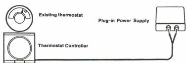
Continue to attach the wire along the baseboard to the nearest wall outlet. Cut the wire to the proper length and strip off the insulation to expose about 1/2" bare ends. Connect the ends of the wire to the screw terminals on the plug-in power supply by wrapping the wire under the screw heads and tightening the screws.
