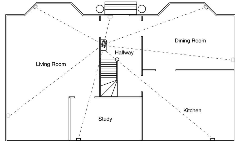
Choose a location for the Security Console which is as central as possible in the house, while providing access to a modular telephone jack and an AC outlet. The Console may be placed on a shelf or table, or may be wall mounted.
