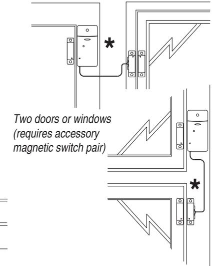
*Note when you add a magnetic switch to a sensor you can register it with the console as its own zone, e.g., the sensor itself can be zone 1 and the extra magnet zone 2. See previous page.*
