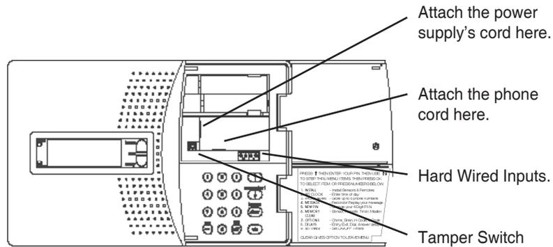
Open the lid on the Console and attach the power supply's cord to the connector labeled power supply (see above). Plug the power supply into any convenient (unswitched) AC outlet.
