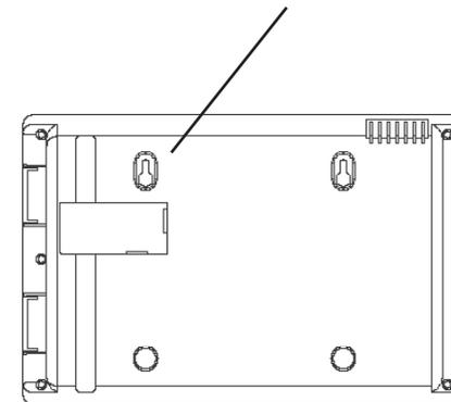
If you don't want to wall mount the console, you can insert the included rubber plugs into the two slotted mounting holes so as to tilt the console slightly forward for better viewing of the display.
