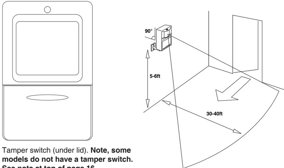
Tamper switch (under lid). **Note, some models do not have a tamper switch. See note at top of page 16.**
