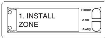
Press the number of the zone you desire (just as if you were going to register the Door/Window Sensor into that zone) but instead of registering the Door/Window Sensor, press CLEAR on the Console's keypad. The display asks you to confirm the deletion:
