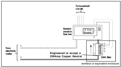
The X-10 PRO 3-phase 250A Signal Blocking Coupler is designed to attenuate (at a rate of 30:1) X-10 power line carrier signals from crossing from one household to another via the AC wiring. The coupler/blocker is installed between the meter and the breaker panel, using the Copper Neutral between the two. The unit may be used in single, dual or three phase installations. For best results a PZZ01 should be installed at both homes experiencing the signal crossings.
