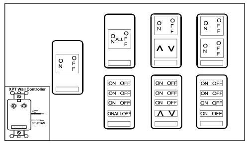
The XP Keypads are designed to operate when attached to an XPT Wall Controller (see insert above). There are seven possible KEYPADS to choose from, allowing multiple control solutions from various locations.
