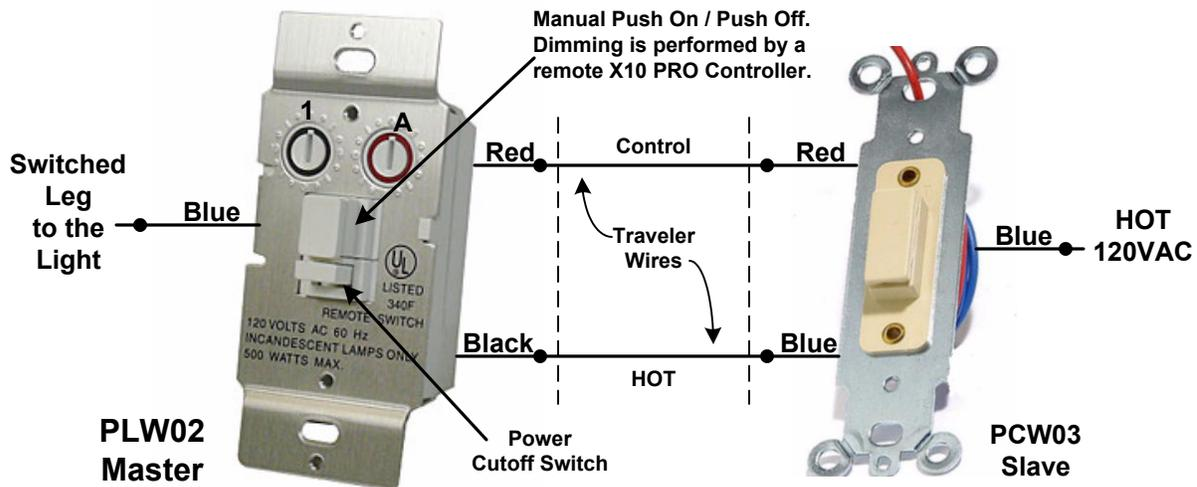
**Description:** The PLW02 3-Way Toggle Style Wall Dimmer Switch Kit is designed to control incandescent bulbs (only) with a rating of 40 to 500W. A pushbutton is provided for local On/Off control on the Master and a single push button on the Slave Switch provides On/Off. A Power Cutoff Switch located directly below the Local On/Off Pushbutton is provided for bulb changing. Both switches should line-up for normal operation. Dimming is provided by an X10 Remote Control only.
