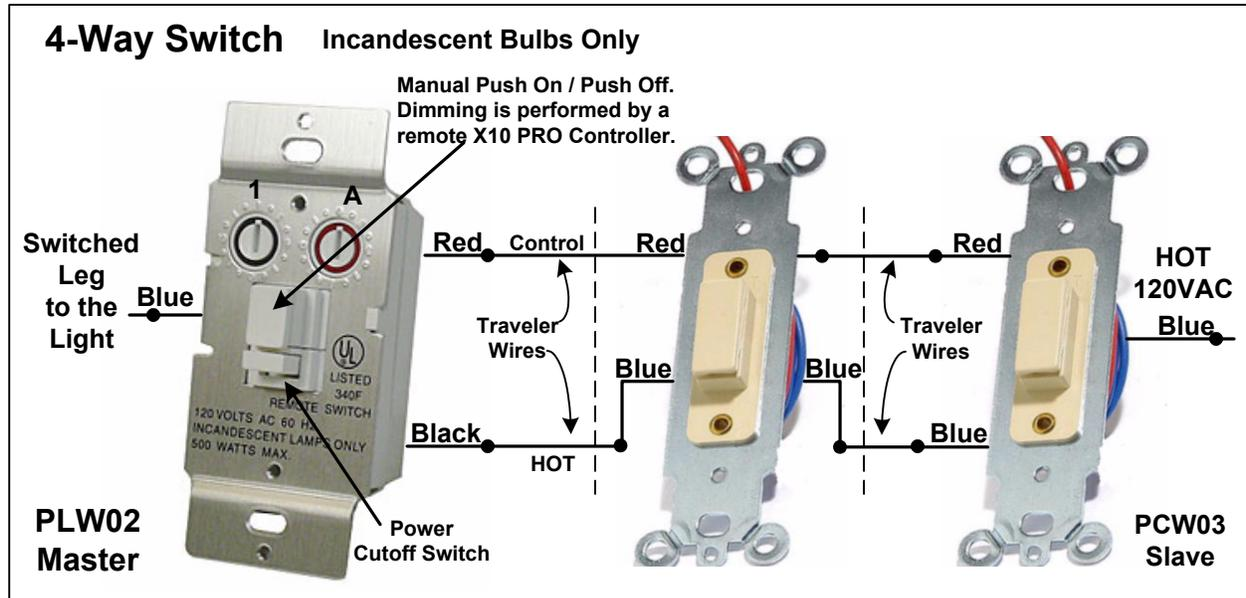
**Description:** The PLW02 3-Way Toggle Style Wall Dimmer Switch Kit is designed to control incandescent bulbs (only) with a rating of 40 to 500W. A pushbutton is provided for local On/Off control on the Master and a single push button on the Slave Switch provides On/Off. A Power Cutoff Switch located directly below the Local On/Off Pushbutton is provided for bulb changing. Both switches should line-up for normal operation. Dimming is provided by an X10 Remote Control only.
