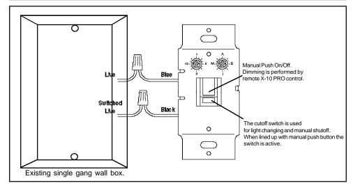
The Wall Dimmer Module is designed to control incandescent loads with a rating of between 40W and 500W. Lamps rated below 40W may flicker or operate erratically. A pushbutton is provided for local on/off control. A power cut-off switch located directly below the local on/off pushbutton is provided for bulb changing. Both switches should line up for normal operation.
