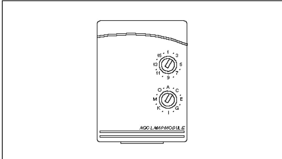
The AGC Lamp Module incorporates an advanced X-10 powerline circuit design which allows the module to operate in adverse environments. The principal advantages are greater sensitivity and better noise rejection. These modules are recommended for larger installations, installations where noise generating equipment such as electric motors etc. are operated nearby and where reliability of operation is paramount.
