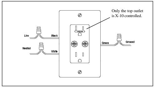
The Wall Receptacle Module is designed to control unrestricted loads up to 15Amp. It provides two outlets, one X-10 controlled (upper) and one which is always on (lower). A trim plate is included to complete the installation.
